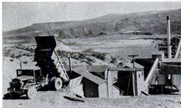
Conversion of rock into oil begins as a dump truck empties shale into a hopper that feeds it to the first of a series of crushers. Photos here show Bureau of Mines' Colorado plant.
