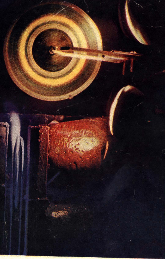
ION ENGINE at NACA lab spins a tiny turbine ( right ). The purple jet of ions, created by high voltage electricity, is accelerated out rear of engine by
