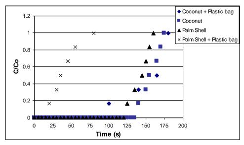
Fig. 4. Breakthrough curve vs time for oil palm shell and coconut shell char, and both chars mixed with plastic bag.
