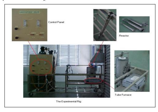
Fig. 1. The Experimental rig for producing carbon adsorbent
