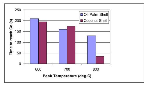
Fig. 3. Time to reach Co for chars of oil palm shell and coconut shell at varies peak temperature
