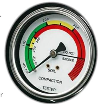
A penetrometer helps to identify the compaction profile and the depth of the restrictive layers. Research has shown that root growth (penetration) essentially stops at 300 psi. Penetration resistance is related to soil water content. Ideally, we would take readings during the spring or the fall when the soil is near its field capacity water content, or during the summer after a substantial rain event. **Talk to your sales rep about taking some penetrometer readings on your farm.**
