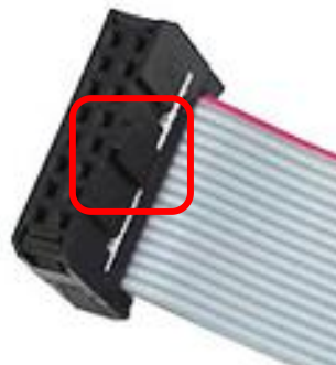
Figure 4 : Protruding portion of connector
