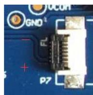
Figure 3 : Connection between DESPI-C03 and front light panel
