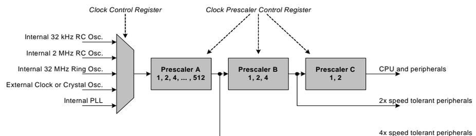
The default setup after a reset is to select the internal 2 MHz RC oscillator and pass the clock signal undivided through all three prescalers. Prescaler A can be used to
