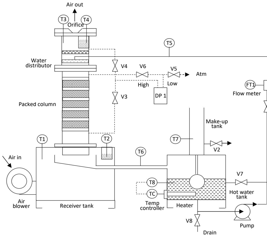
**Figure 1** Schematic Diagram of the Water Cooling Tower
