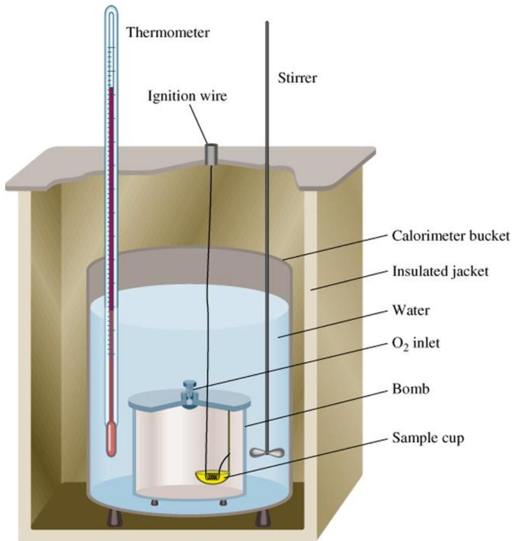
$$q_{\text{sys}} = q_{\text{water}} + q_{\text{bomb}} + q_{\text{rxn}}$$
