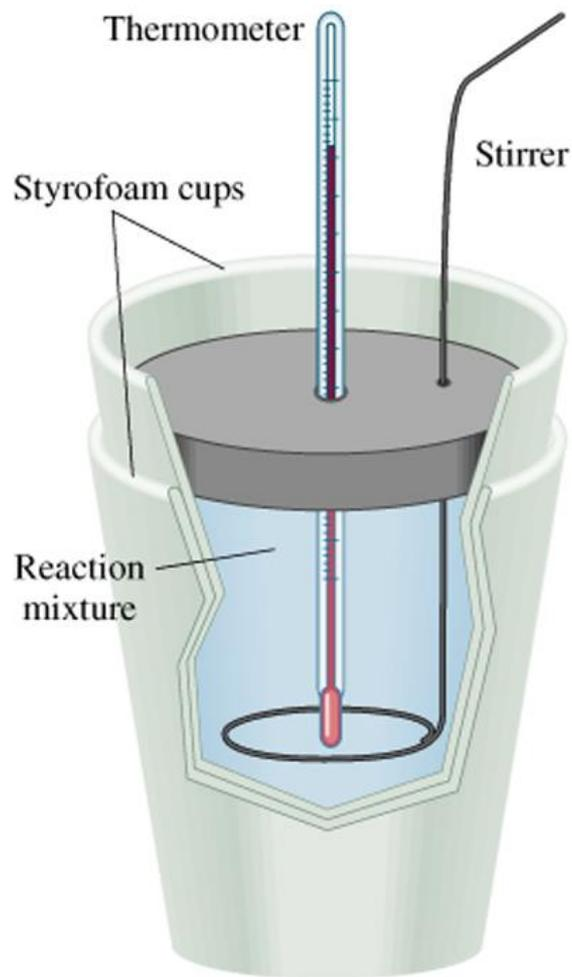
$$q_{\text{sys}} = q_{\text{water}} + q_{\text{cal}} + q_{\text{rxn}}$$
