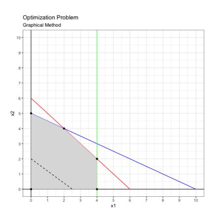
Based on the plot above, the objective function line can be displaced even more to the right.
