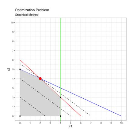
As seen on the plot above, the simplex algorithm final outcome was (2,4), same as the outcome reached using the graphical method. The red dot (i.e. simplex solution) matches the last point the objective function line (i.e. black dashed line) touches before exiting the feasible region, thus, confirming that x1 = 2 and x2 = 4 leads the maximum possible value of z, 28.
