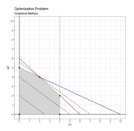
At this point, the objective function line cannot be further displaced to the right because it would exit the feasible region, thus, the optimum solution has been reached at (2,4).
