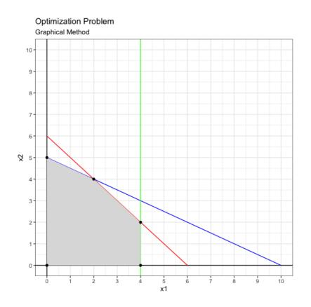
The feasible region above contains all the possible combinations of x1 and x2 that satisfy the given constraints. However, the optimum solution of the problem will be located in one of its corner points, either (0,0), (4,0), (4,2), (2,4) or (0,5).
